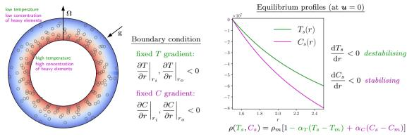
Consider a Boussinesq fluid in a rotating spherical shell of inner radius  $r_i$  and outer radius  $r_o$
