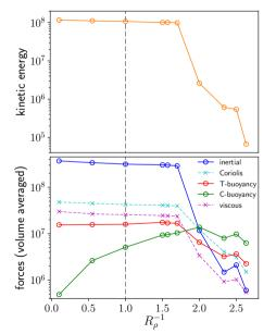
$$\frac{\partial \boldsymbol{u}}{\partial t} + \underbrace{(\boldsymbol{u} \cdot \nabla)}_{\text{inertia}} \boldsymbol{u} + \underbrace{\frac{2}{Ek} \boldsymbol{\hat{z}} \times \boldsymbol{u}}_{\text{Coriolis}} = -\nabla \Pi + \underbrace{\Theta \, r \, \boldsymbol{\hat{r}}}_{\text{buoyancy}} - \underbrace{\xi \, r \, \boldsymbol{\hat{r}}}_{\text{ompositional buoyancy}} + \underbrace{\nabla^2 \boldsymbol{u}}_{\text{viscout}}$$
