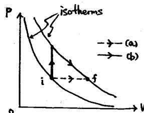
4. (SB 24) (a)  $P_i V_i^\gamma = P_f V_f^\gamma$
