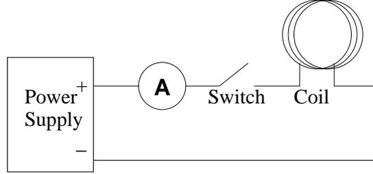
FIG. 1: The circuit used to generate magnetic field in the experiment
