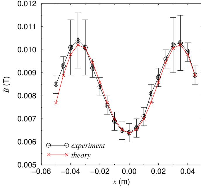
FIG. 5:  $B$  versus  $x$  for two circular coils with current flowing in the same sense
