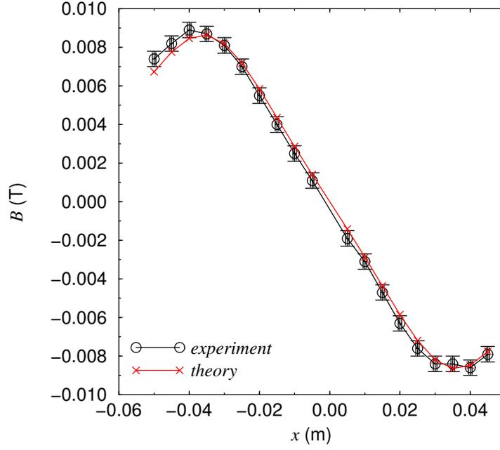
FIG. 6:  $B$  versus  $x$  for two circular coils with current flowing in the opposite sense
